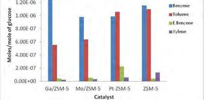
BTEX yield with metal incorporated ZSM-5 when glucose is pyrolyzed in the presence of methane (BTEX:benzene, toluene, ethylbenzene, and xylene)
