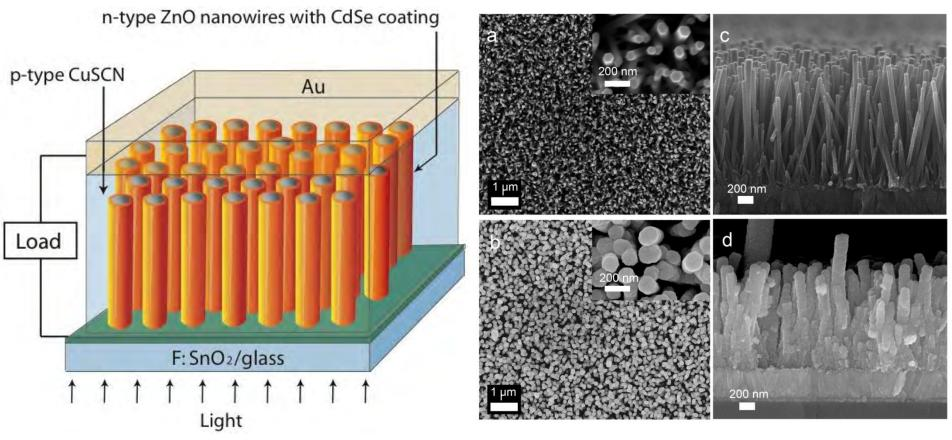
Extremely thin absorber (ETA) solar cells have been fabricated. Light is absorbed in the CdSe coating, where the photoexcited electron is injected into the ZnO and the hole is injected into the CuSCN.
