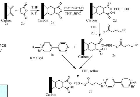
Developed new schemes to covalently attach the organic catalyst to electrode surfaces, which are currently being tested for electrochemical activity.
