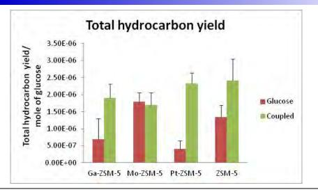
Mo-ZSM-5 is the best catalyst for deoxygenation of pure glucose. When methane is used as the proton donor for deoxygenating glucose, H-ZSM-5 and Pt-ZSM-5 performed better. The analysis shows that the yield of total hydrocarbons are significantly higher when glucose is catalytically pyrolyzed in the presence of methane.
